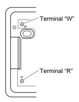
Figure 36 - Thermostat Base Terminal "W" and "R"
